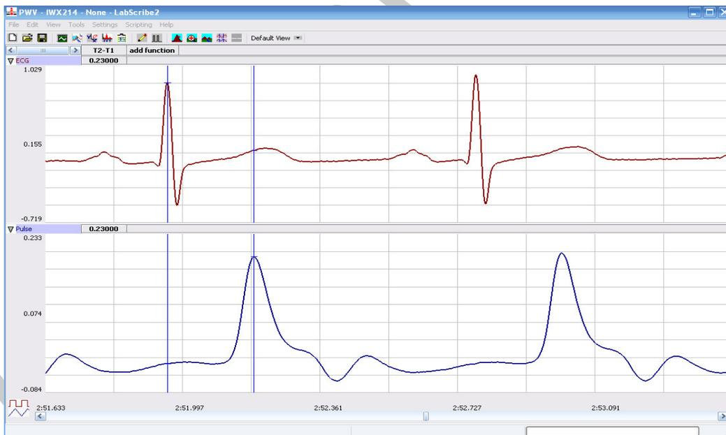
Figure HC-3-L3: An ECG and pulse wave recording shown in the Analysis window. The pulse plethysmograph was placed on the tip of the left middle finger. The time difference ( $T_2-T_1$ ) between the peaks of the R and pulse waves is 230 msec.
