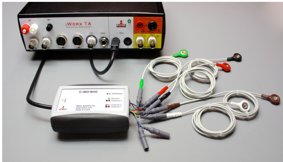
Figure HM-7-S3: A five lead EMG cable connected to an IXTA.
