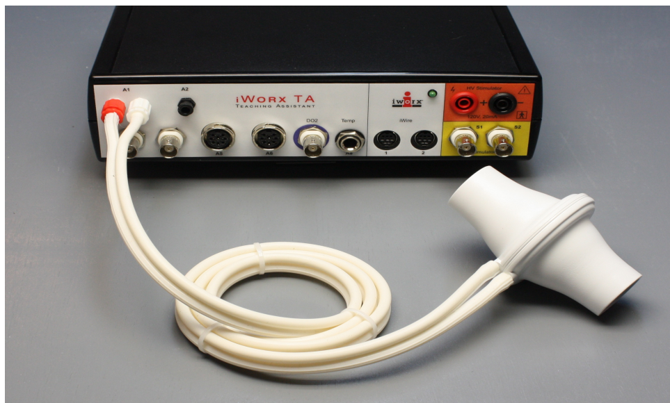
Figure HS-2-S2: The flow head connected to the internal spirometer of the IXTA unit.
