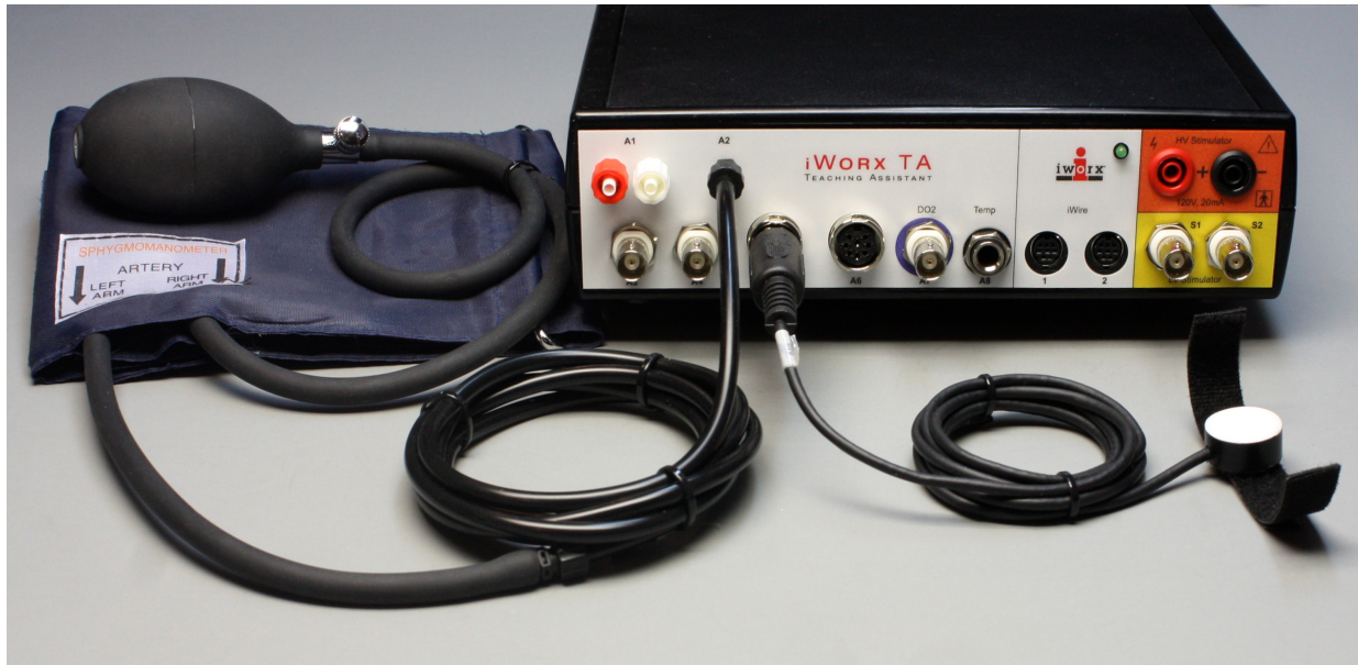
Figure HC-2-S3: The PT-104 pulse transducer and the BP-220 non-invasive blood pressure transducer connected to an IXTA.
