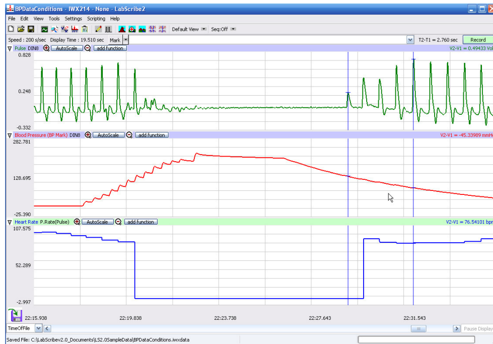
Figure HC-2-L1: The pulse wave, the cuff pressure, and heart rate recorded before, during, and after the occlusion of the brachial artery. Pulses disappear as the pressure in the cuff exceeded the pressure in the artery. As the pressure in the cuff is released, the pulse wave reappears.
