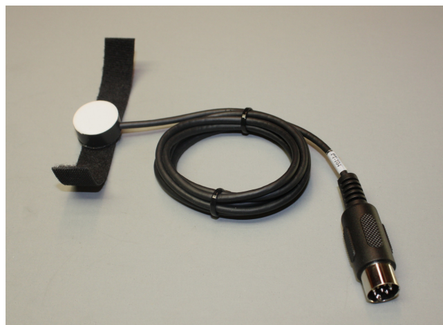
Figure HC-2-S2: The PT-104 pulse plethysmograph.
