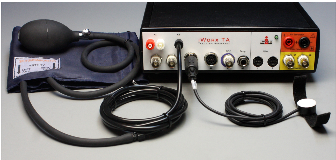
Figure HC-1-S3: The PT-104 pulse transducer and the BP-220 non-invasive blood pressure transducer connected to an IXTA.
