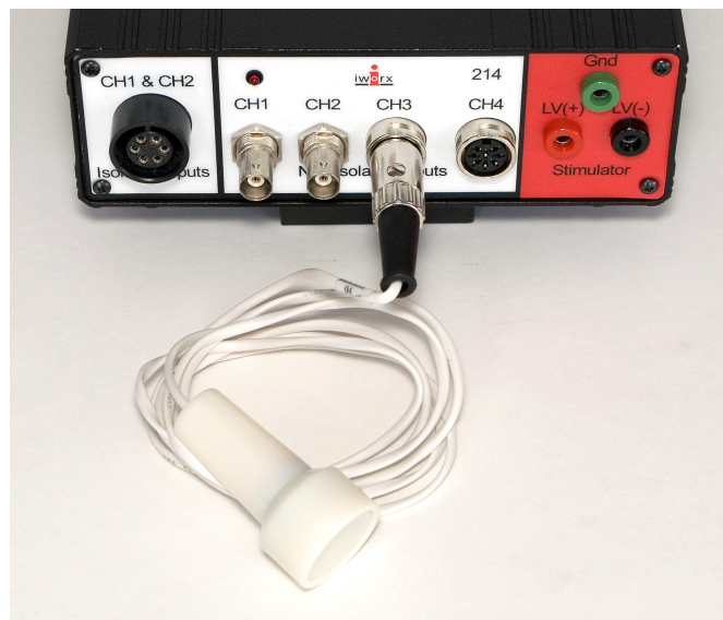
Figure HN-1-L1: The EM-100 event marker connected to an IWX/214.
