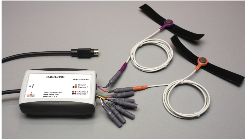
Figure HP-8-S2 The C-ISO-B3G galvanic skin response amplifier.
